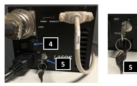
If the Argon Laser (black box) is required (458, 488, 514 nm) press the switch button to ON [4] and turn the key (horizontal= ON) [5]
